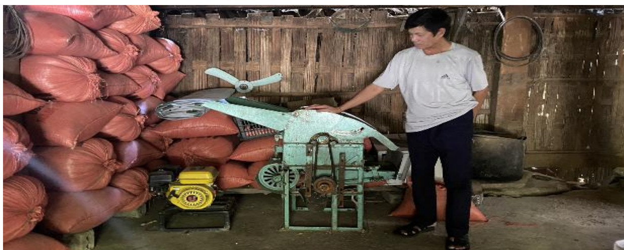
Photo 8: Improved rice thresher supported by the project for Hop 1 village, Ban Lang commune
